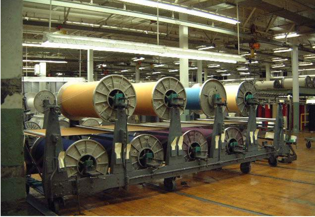
Figure 6. Slasher creel loaded with beam-dyed yarns for a warp-striped fabric
