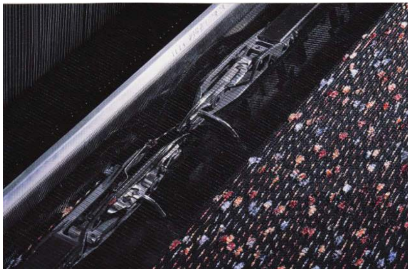
Figure 19. Double rigid rapier machine (courtesy of Dornier)
