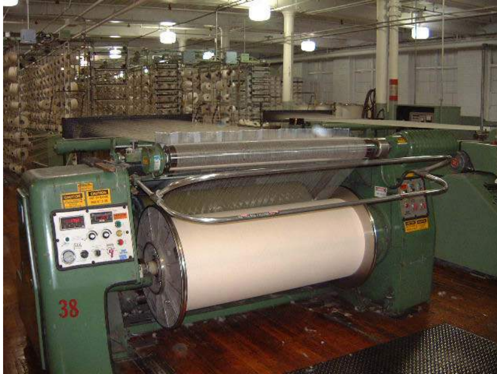
Figure 2. Direct warping from yarn packages to a section beam
