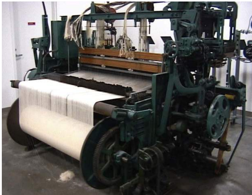
Figure 15. Rear view of a shuttle loom
