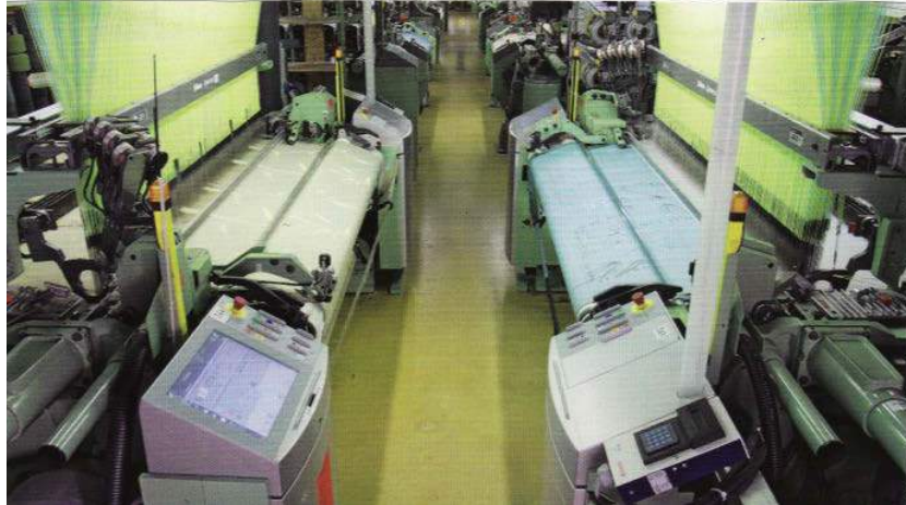
Figure 17. Rigid rapier machines with Jacquard shedding (courtesy of Dornier)
